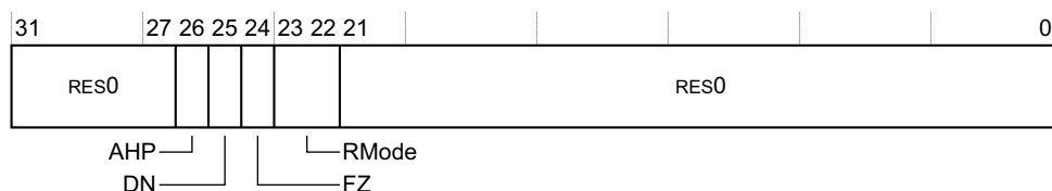
Figure 14-1 FPCR bit assignments
