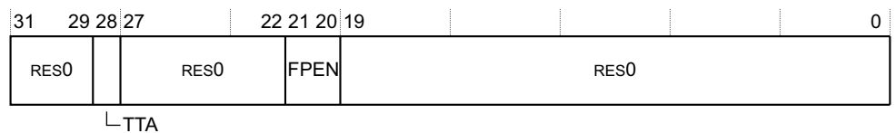
Figure 4-29 CPACR_EL1 bit assignments
